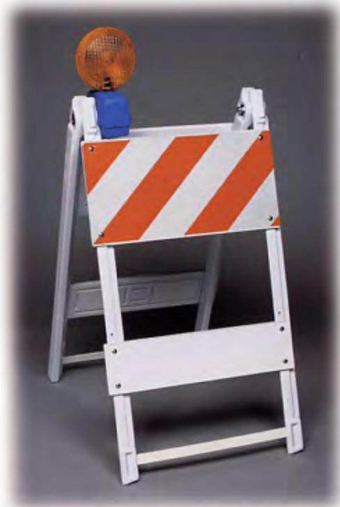
Type I Barricade with 12" x 24" top panel and 6" x 24" bottom panel. (Optional breakaway sand bag bar pictured above)
