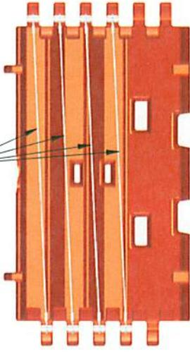
CUT AWAY VIEW DISPLAYING INTERNAL MOLDED IN BARRIER CABLES
