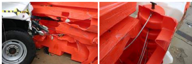
Four Cables, Preventing Vehicle Breaching
