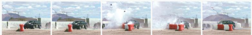
TraFiX Water-Cable Barrier® TL-2 Impacted by a 2,505 lb. (1,113 kg) KIA Rio at 44 MPH (70 KPH)
