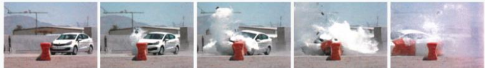
TrafFix Water-Wall LCD impacted by a 2,505 lb. (1,113 kg) KIA Rio at 44 MPH (70 KPH)
